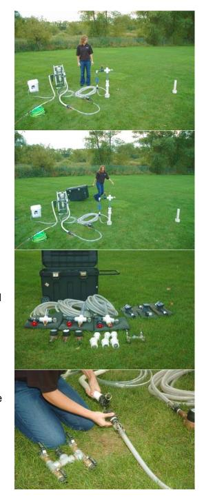
Install the 1 x 4 manifold with the camlock connectors.
