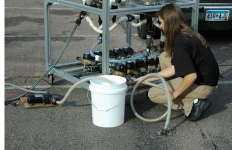
Connect the 20' clear vinyl amendment hose directly to one of the Dosmatic™ feeders and put the other end into the 5-gallon pail. Connecting directly to the pump makes for easier cleanup than using the vinyl Y-hose that connects the two Dosmatic. This step is necessary to circulate antifreeze in the pump end of the Dosmatic. Pour 3 gallons of propylene glycol into the pail to start. You may need to add more glycol as the process continues.
