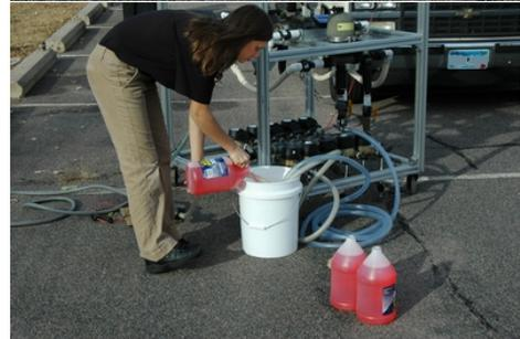
The 12v pump does not have the capacity to operate both Dosmatic feeders at the same time. Trace out the 1" white spa hoses (they cross) and use the 1" ball valves to isolate the pump that is NOT connected to the amendment hose.
